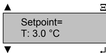
Setpoint = 3.0°C shows the cooling set-point temperature. By pressing the "▲" and "▼" keys, the temperature set-point can be altered. A value 3.0° C is the default value. The "⏏" key takes you to the next level down in the menu.
