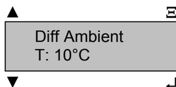
Diff Ambient T:10°C determines the difference between ambient and cooler temperature. In this example, the difference is 10°C. This difference indicates the degree of drying and the 10°C (preset in the factory) may not be reduced or the unit will switch "off". Below this point there is a risk that even after the condensate key displays "off", the selected temperature <10°C will not be reset.
