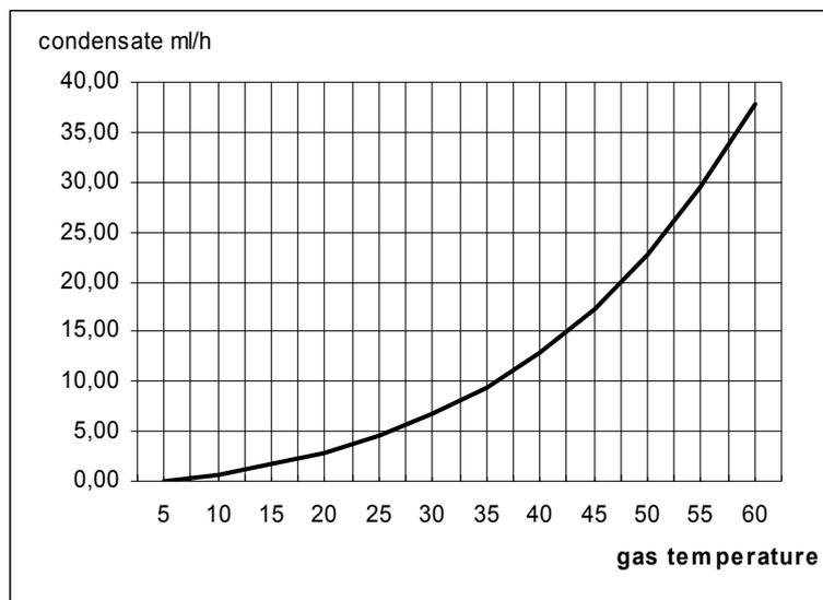
This graph shows the condensed water volume at 250ml/h gas at a dew point of 3°C
