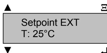
Setpoint EXT T:25°C displays the cooling fan activation temperature and the fan switches on if the ambient temperature exceeds this value. The "⏏" key takes you to the next level down in the menu.
