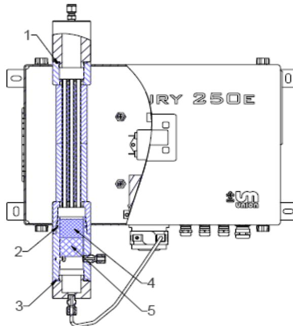
Figure 6 : Capillary cooler with filter unit
