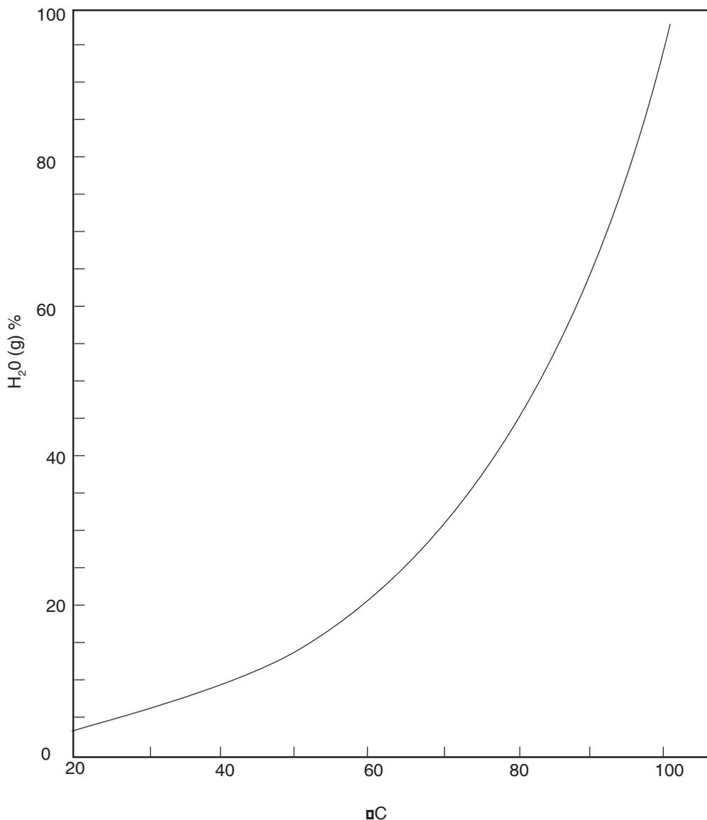
This graph shows water vapour condensation point from 0 to 100°C
