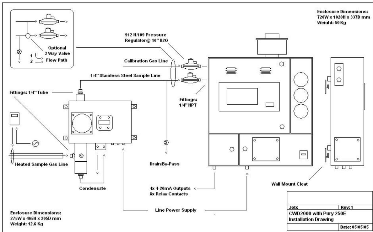
Figure 2 : Typical gas connection diagram
