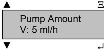
Depending on the dew point of the gas, more or less liquid condensate will be removed after drying. The volume of condensate removed is indicated in ml/h and the accumulated condensate volume can be calculated by using the tables in Chapter 10, The condensate pump will then automatically discharge the required volume of condensate from the system, at predetermined intervals.
