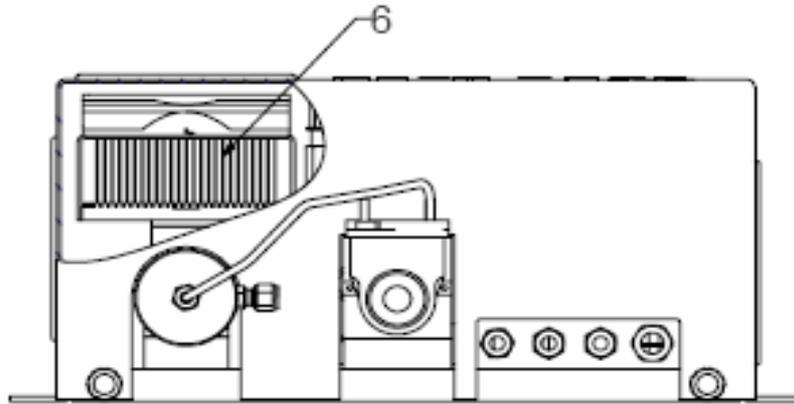
Figure 7 : Cooling block with finned cooling body (6)
