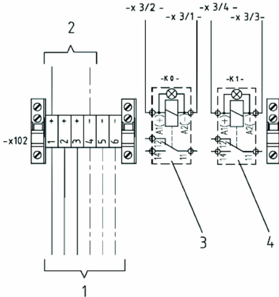
Figure 4 : Internal 24 Volt power supply diagram
