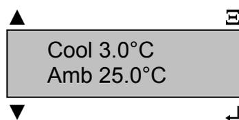
Cool 3.0°C and Amb 25.0°C shows a cooler temperature of 3°C at an ambient temperature of 25°C. The "⏏" key takes you to the next level down in the menu.
